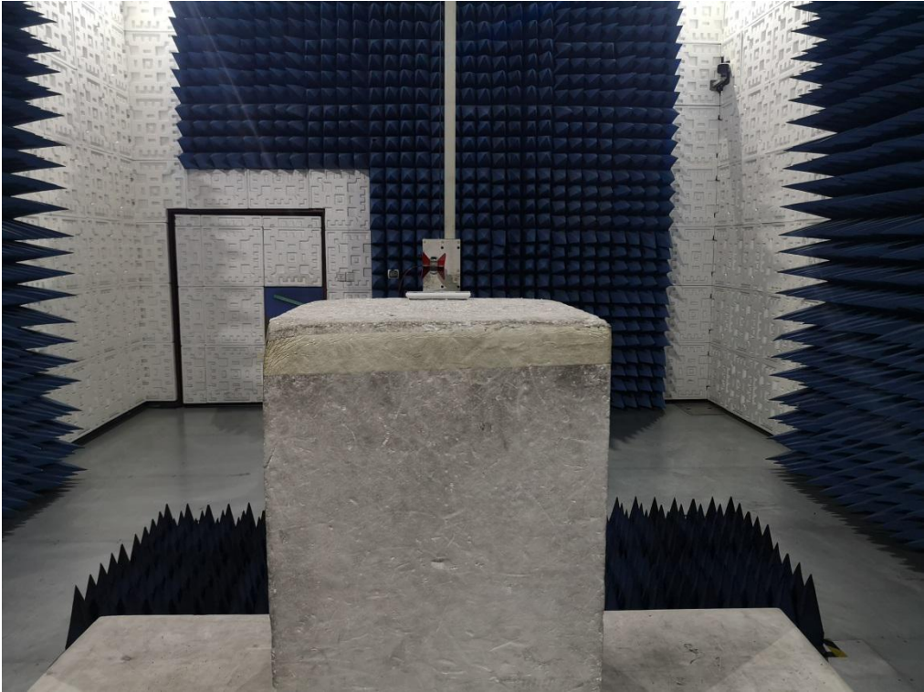
FCC RADIATED EMISSION TEST SETUP-ABOVE 1GHz
