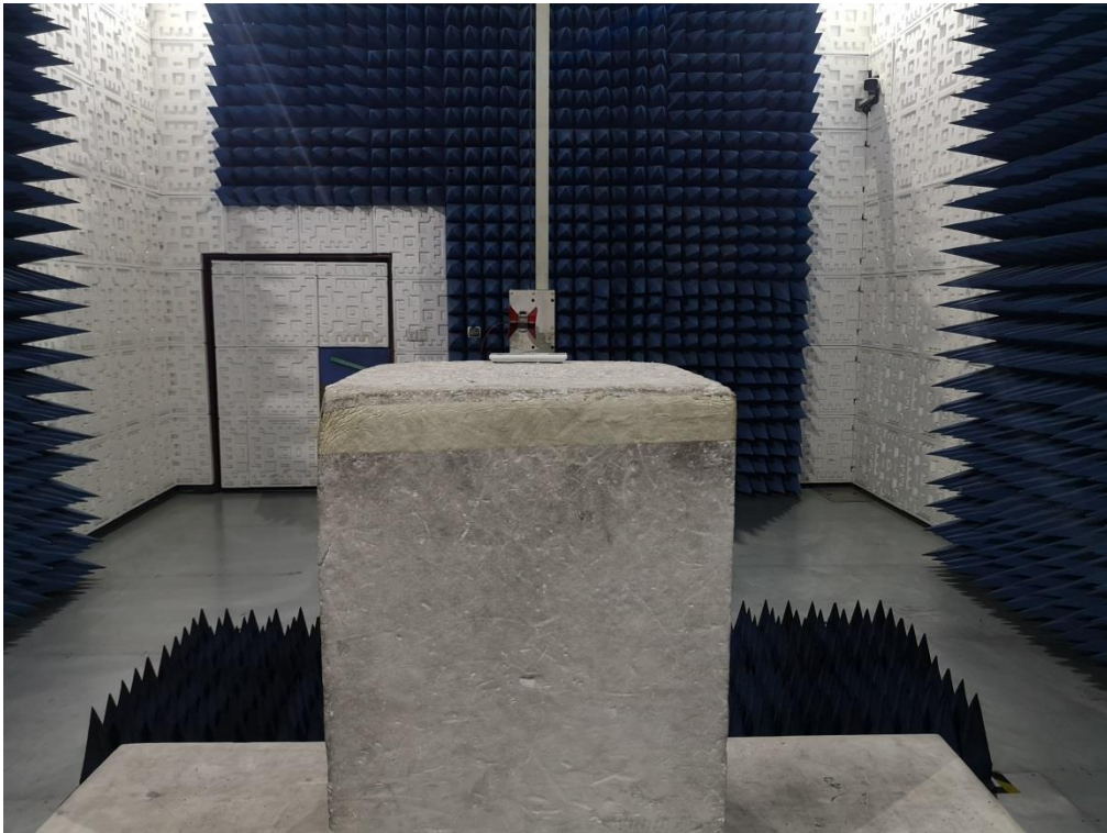
FCC RADIATED EMISSION TEST SETUP-ABOVE 1GHz
