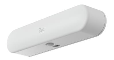
RTJSD02 counting sensor receives thermal IR energy from objects through its thermopile array to detect people passing through. The sensor can calculate the number of passing people and their direction of travel.
