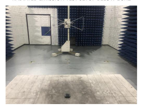
RADIATED EMISSION TEST SETUP ABOVE 1GHZ
