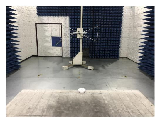
RADIATED EMISSION TEST SETUP ABOVE 1GHZ
