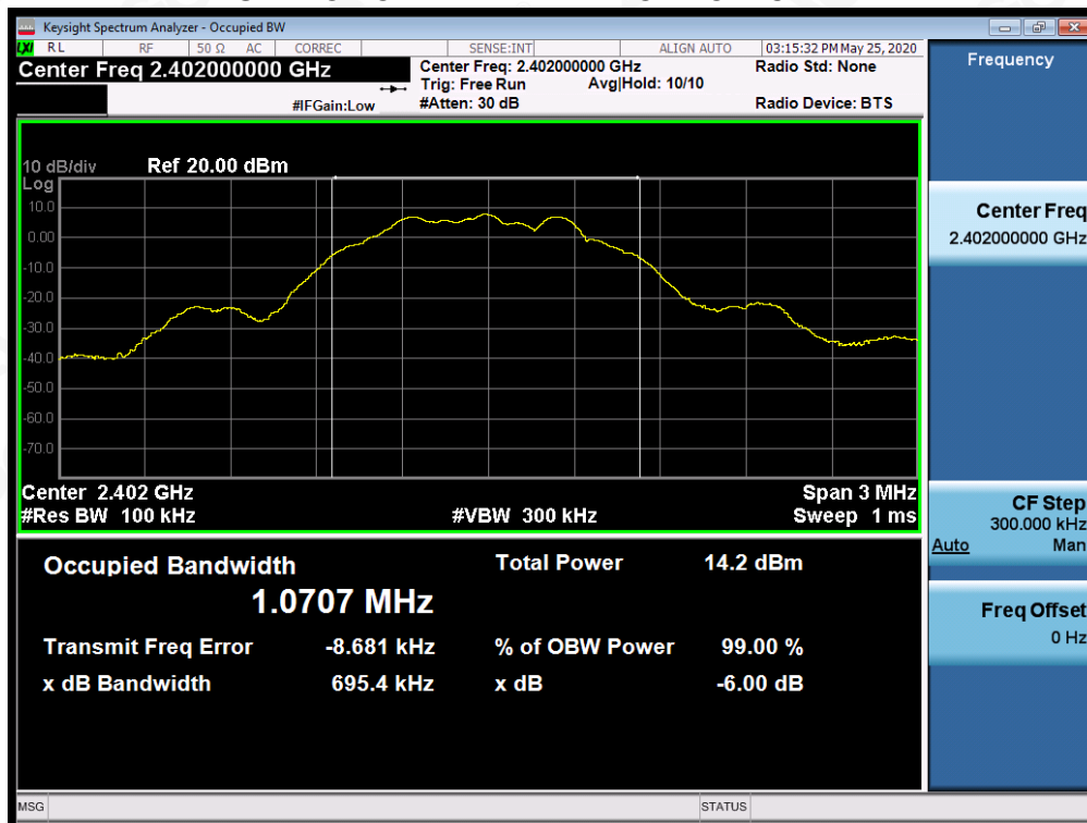
TEST PLOT OF BANDWIDTH FOR LOW CHANNEL
