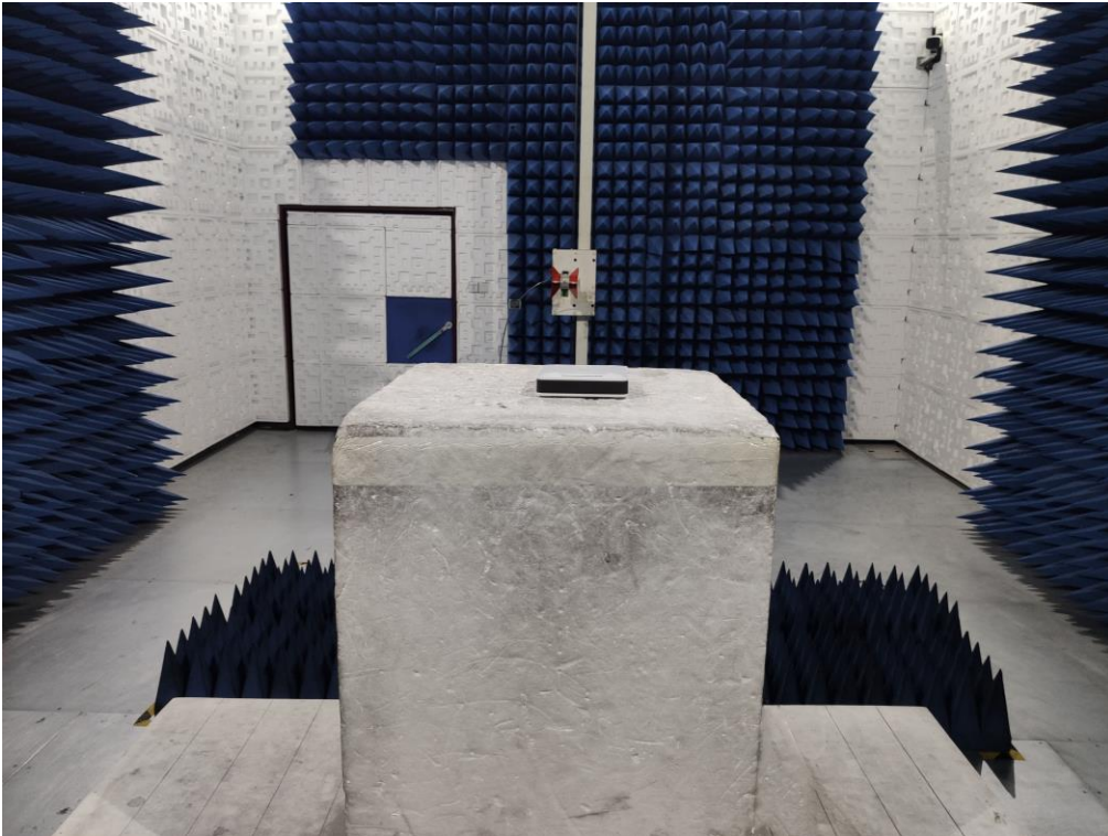
RADIATED EMISSION TEST SETUP ABOVE 1GHZ
