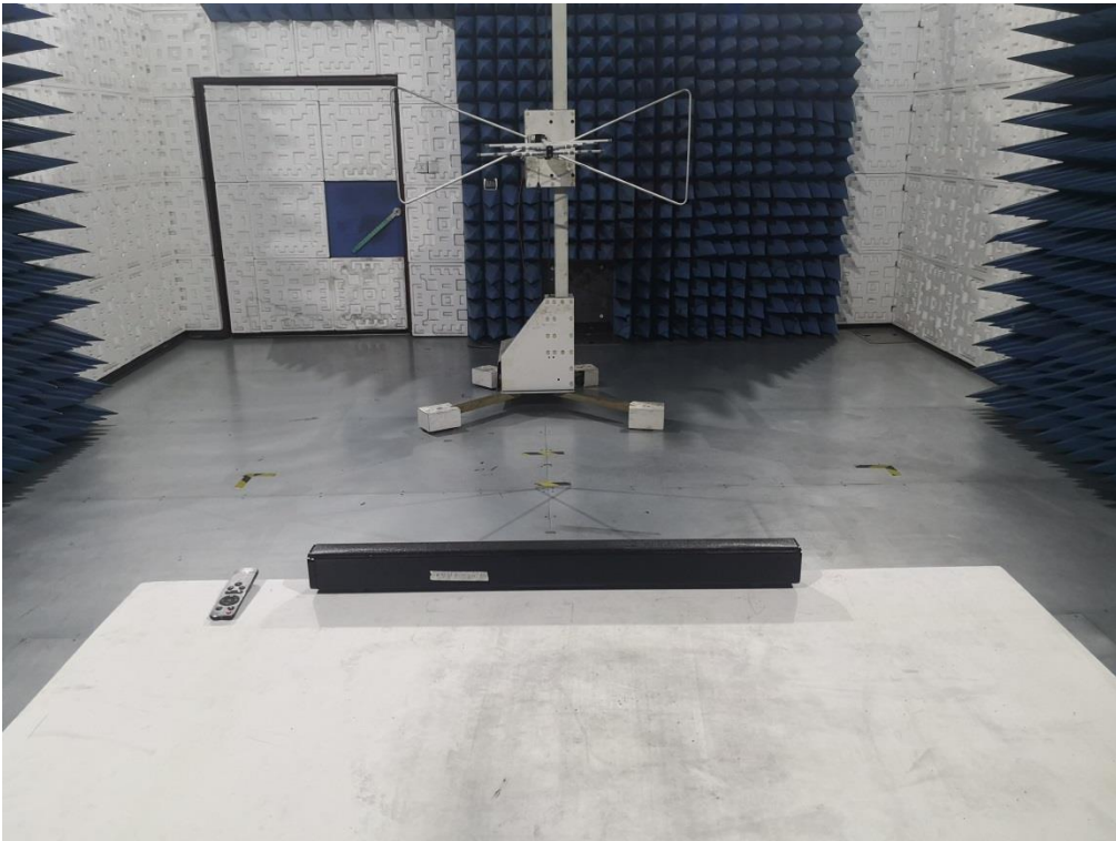
RADIATED EMISSION TEST SETUP ABOVE 1GHz
