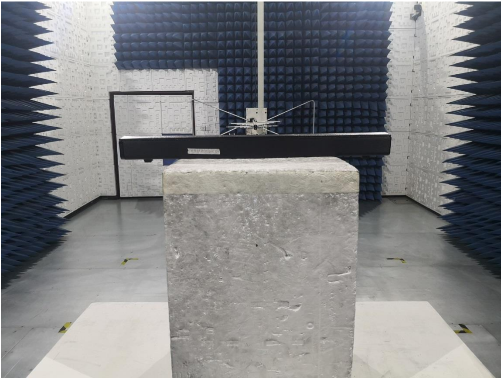
RADIATED EMISSION TEST SETUP ABOVE 1GHz
