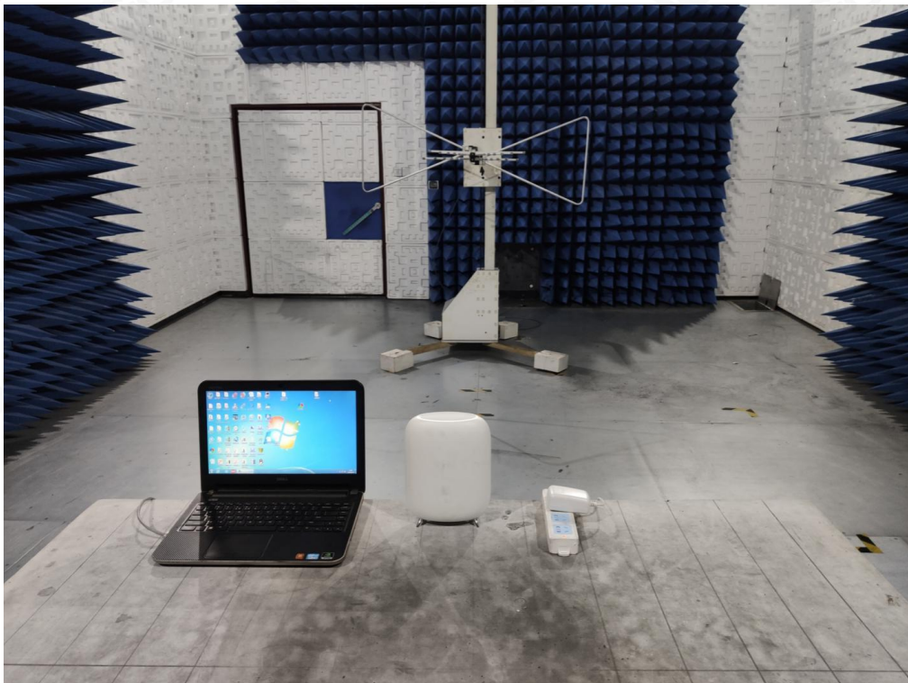
FCC RADIATED EMISSION TEST SETUP BELOW 1GHZ
