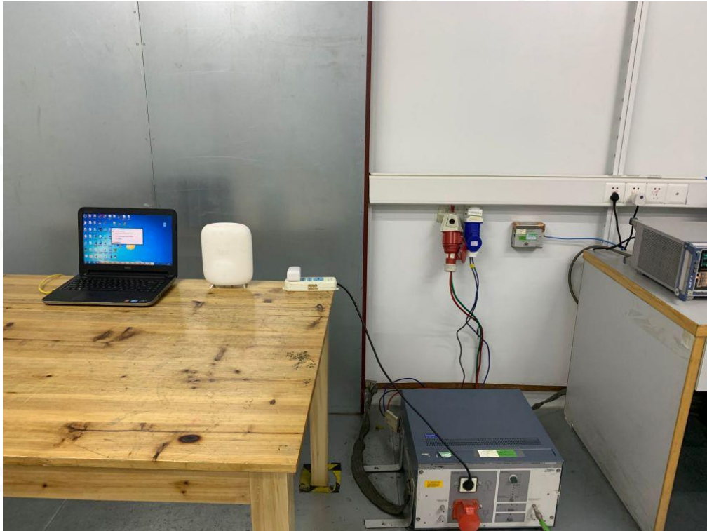
FCC RADIATED EMISSION TEST SETUP BELOW 1GHZ
