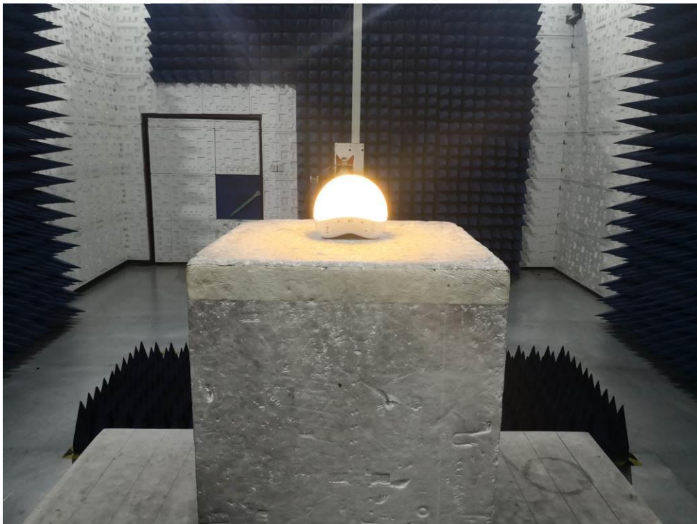
FCC RADIATED EMISSION TEST SETUP ABOVE 1GHZ
