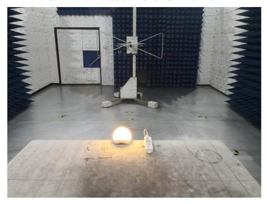
FCC RADIATED EMISSION TEST SETUP ABOVE 1GHZ
