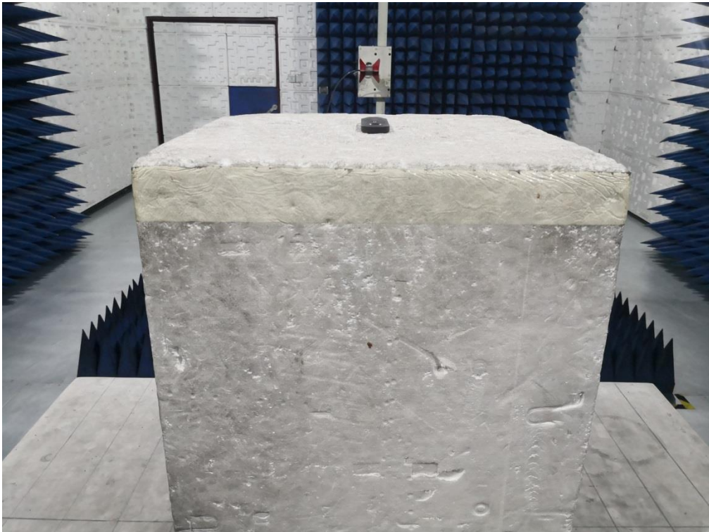
RADIATED EMISSION TEST SETUP ABOVE 1GHZ
