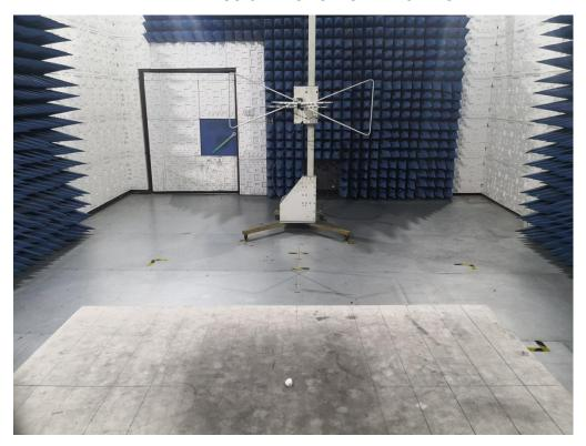
RADIATED EMISSION TEST SETUP ABOVE 1GHz
