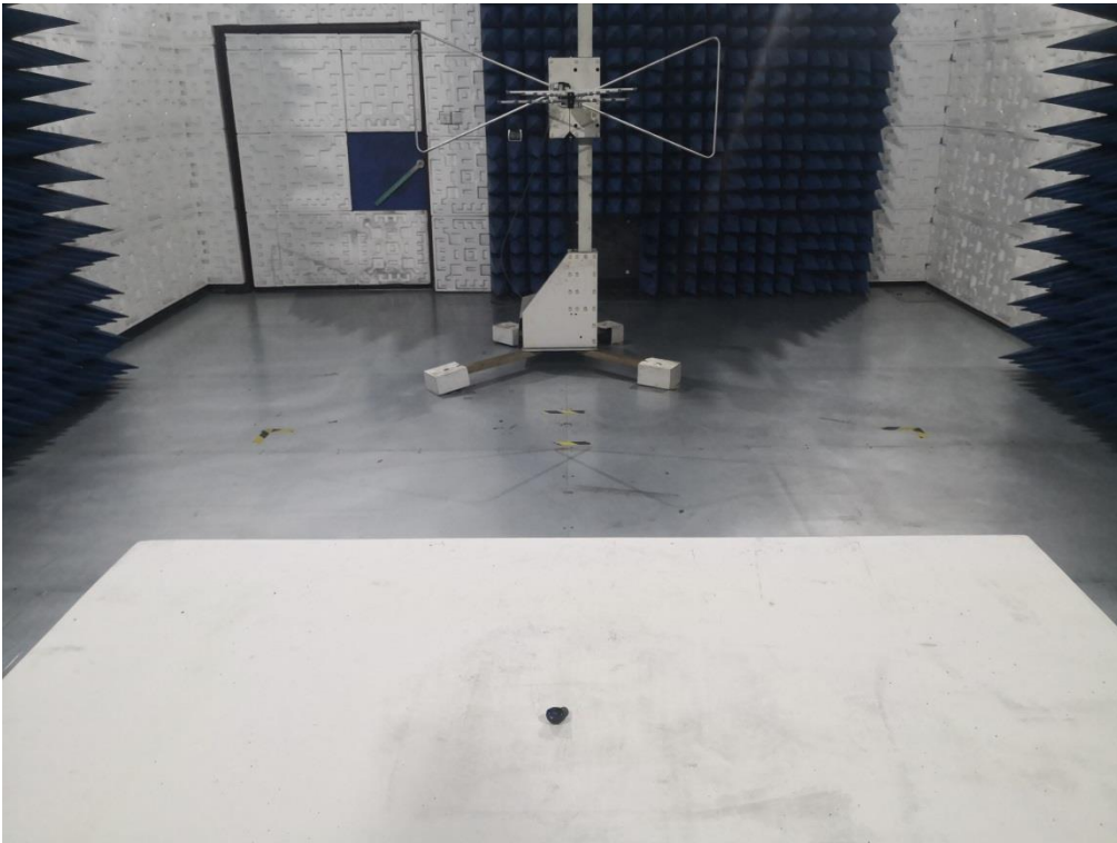
RADIATED EMISSION TEST SETUP ABOVE 1GHz
