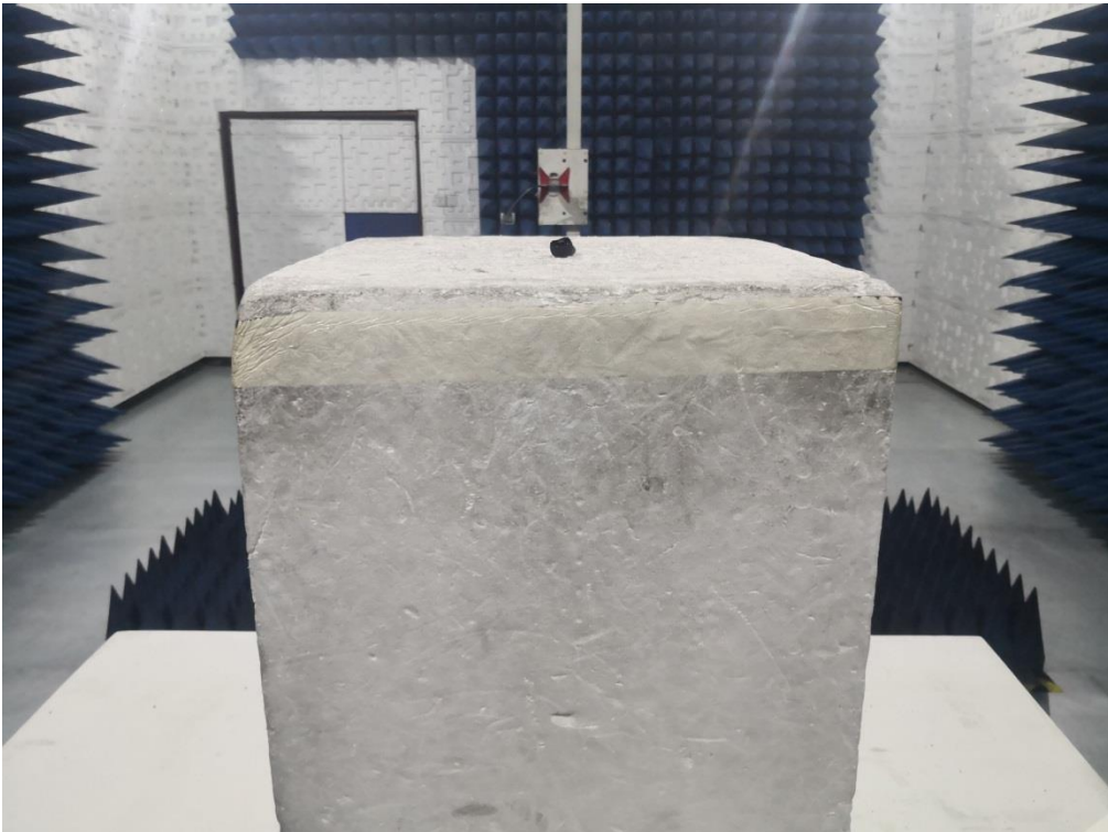
RADIATED EMISSION TEST SETUP ABOVE 1GHz
