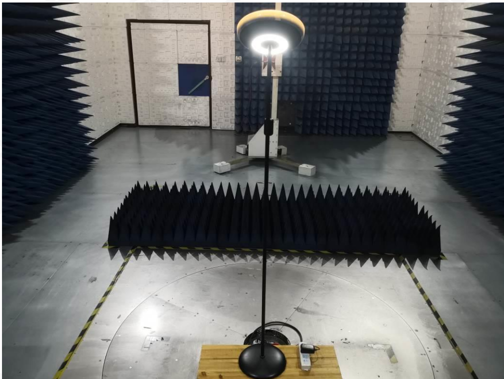
FCC RADIATED EMISSION TEST SETUP ABOVE 1GHZ
