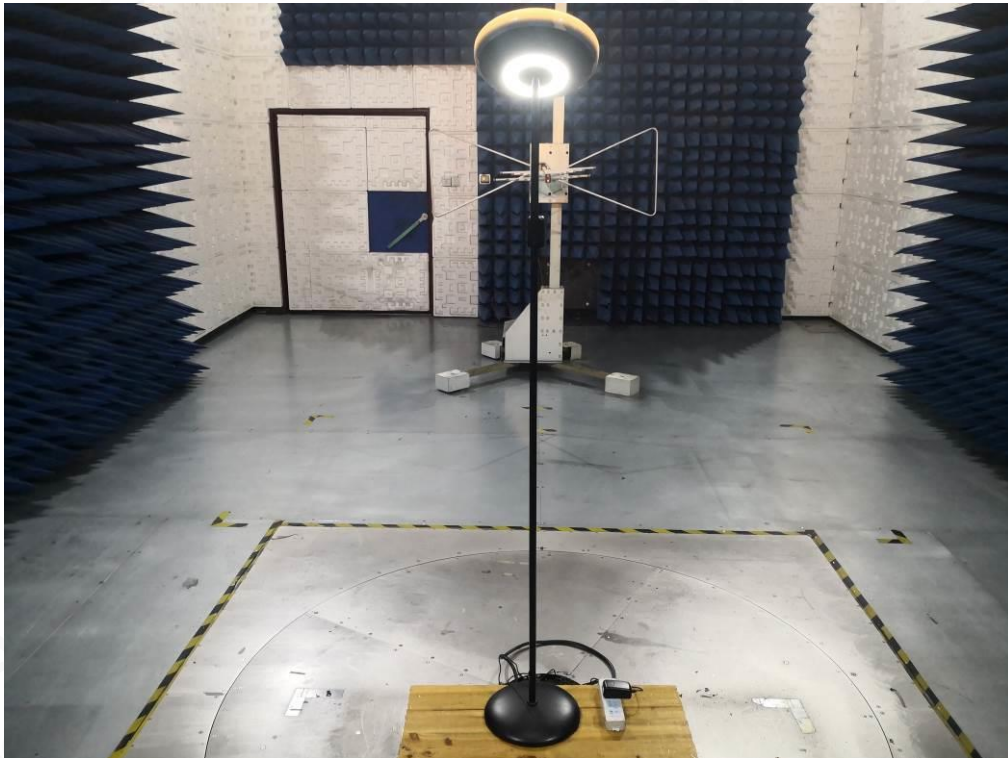
FCC RADIATED EMISSION TEST SETUP ABOVE 1GHZ
