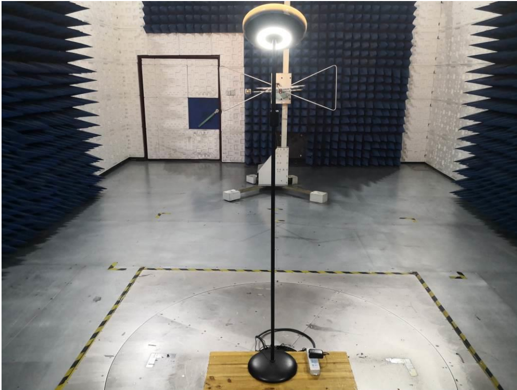
FCC RADIATED EMISSION TEST SETUP ABOVE 1GHZ
