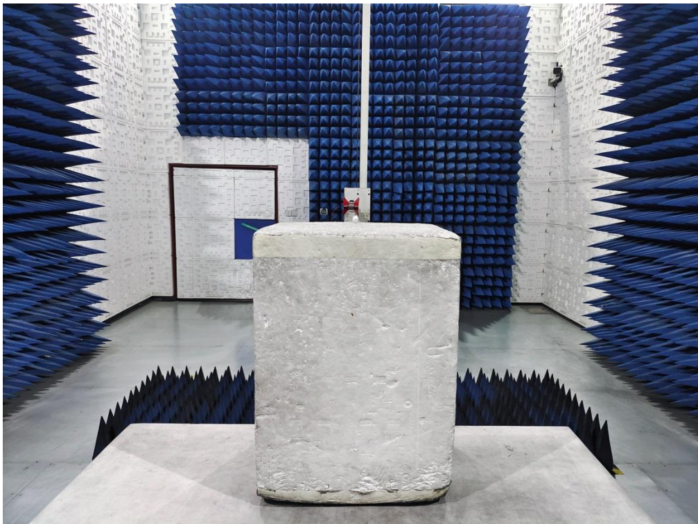
RADIATED EMISSION TEST SETUP ABOVE 1GHz
