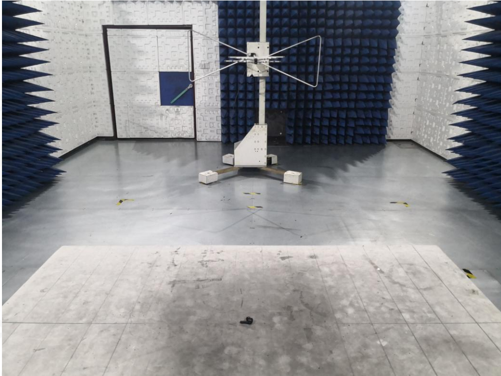
RADIATED EMISSION TEST SETUP ABOVE 1GHZ
