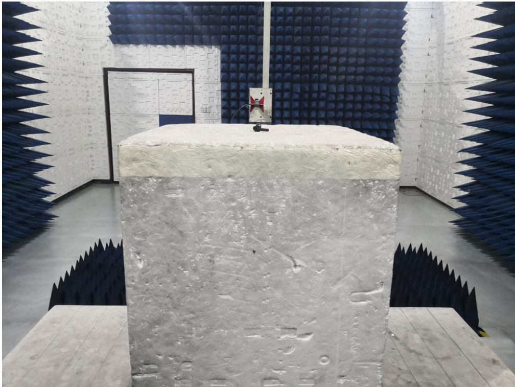
RADIATED EMISSION TEST SETUP ABOVE 1GHZ
