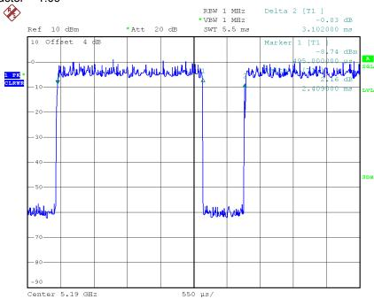
Note: The EUT was programmed to be in countinously transmitting mode and the transmit duty cycle is not less than 98 %, so, the output power and power density should be cacluated as Output Power = Measured power + Duty factor
