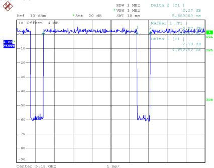
Note: The EUT was programmed to be in countinously transmitting mode and the transmit duty cycle is not less than 98 %, so, the output power and power density should be cacluated as Output Power = Measured power + Duty factor
