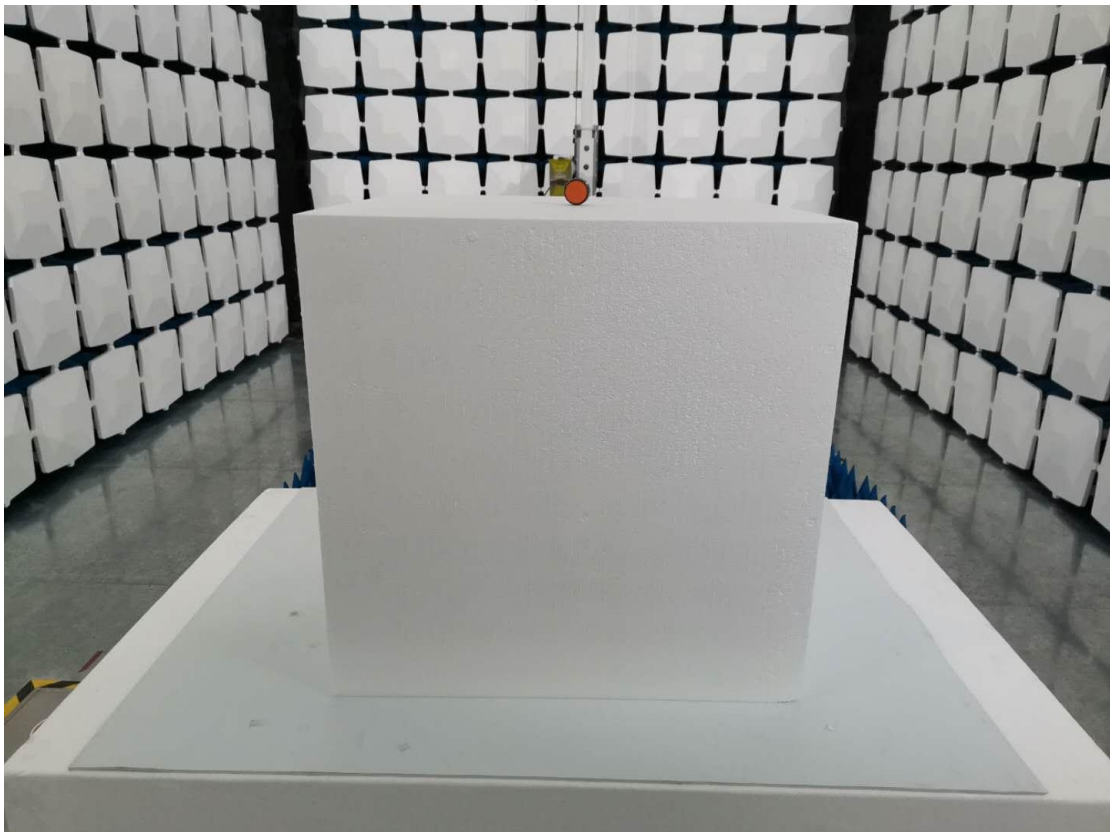
Above 1GHz for radiated emission test setup
