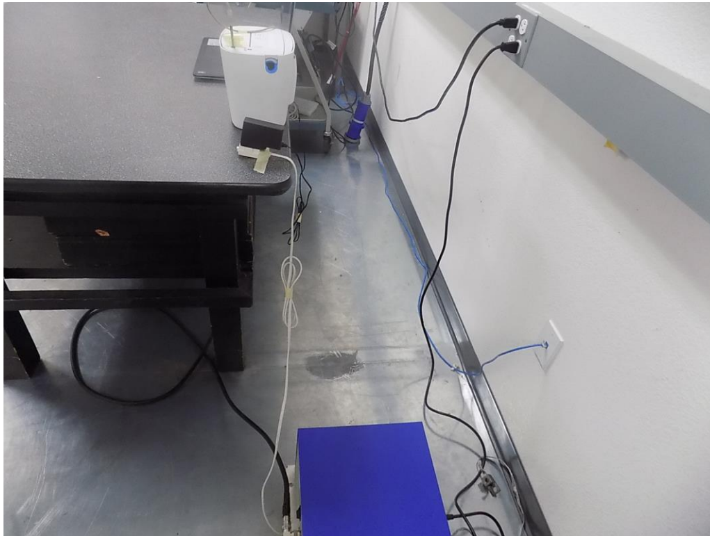
Figure 2: Test Setup for Conducted Emissions – Back (AC Mains)
