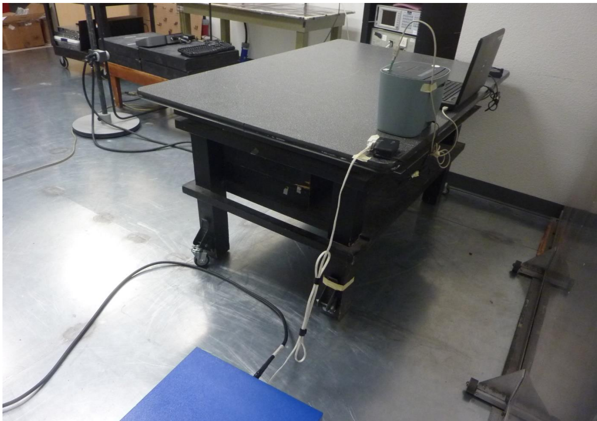
Figure 2: Test Setup for Conducted Emissions – Back (AC Mains-RFID)
