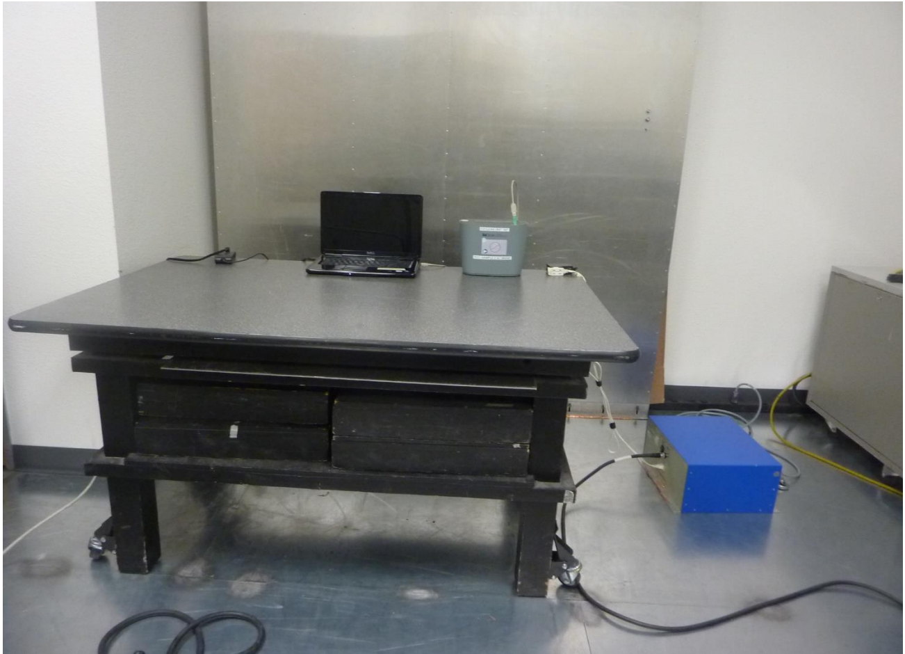
Figure 1: Test Setup for Conducted Emission – Front (AC Mains-RFID)
