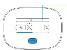
**STEP 2:** At the end of the Fresh Air Cycle, the **Cycle Complete** icon will light up **green**. You can now open the Lid and remove your mask and hose.
