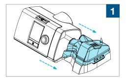
Remove the reservoir from the CPAP machine.
