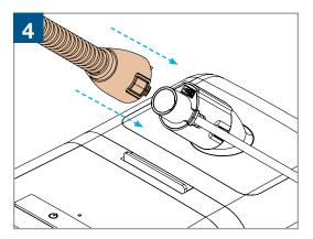
Close the reservoir lid and attach the CPAP hose to the Hose Port Adapter.
