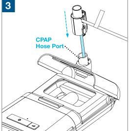
Guide the Adapter Tube down into your reservoir through the CPAP Hose Port, making sure that the Adapter Tube passes into the reservoir opening and rests near the bottom of the reservoir under the water level. Attach the Hose Port Adapter to the CPAP Hose Port.
