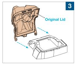
Install the **Original Lid** to the reservoir base by inserting the hinge pins into the notches on the reservoir base. If needed, insert one hinge pin at a time and gently flex the lid to snap it in place.
