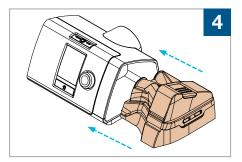
Close the **Original Lid** and install the reservoir back into your CPAP device.
