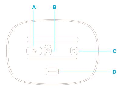
**NOTE:** There is no power button on your SoClean 3. The device is connected to power and "on" when the Power Adapter is plugged into your SoClean 3 and the AC wall socket.
