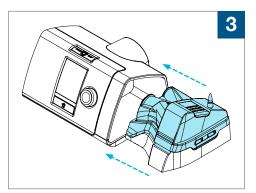
If needed, fill your reservoir with distilled water. Close the **Reservoir Lid Adapter** and insert the reservoir into your CPAP unit like you normally would.
