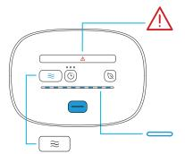
During the Disinfect Cycle cancellation, the **Fault/Unable to Run** icon will illuminate **red**, indicating the Lid is locked and the **Cycle Start** button will illuminate **blue**. The **Progress Bar** on the Control Panel will **flash blue** while the cycle cancellation is in progress.
