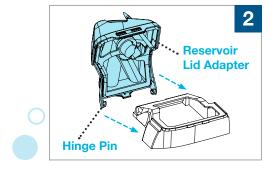
Install the **Reservoir Lid** Adapter to the reservoir base by inserting the hinge pins into the notches on the reservoir base. If needed insert one hinge pin at a time and gently flex the **Reservoir Lid** Adapter to snap it in place.
