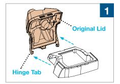
Remove the **Original Lid** from the CPAP reservoir base by opening the **Original Lid** fully, pushing one side of the hinge tab outward and freeing the **Original Lid** from the base.
