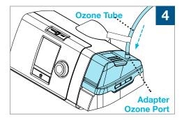
Connect the Ozone Tube to the Reservoir Lid Adapter by pushing the Ozone Tube onto the Adapter Ozone Port.
