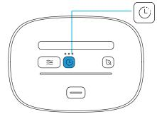
**STEP 1:** With your CPAP mask in your SoClean 3, press the **Cycle Delay** button to select the cycle delay time. The delay button will flash to indicate that the Cycle Delay can be changed.
