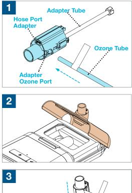
Connect the Ozone Tube from the SoClean to the Adapter Ozone Port.
