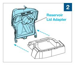
Remove the **Reservoir Lid** Adapter from the reservoir base by opening the **Reservoir Lid Adapter** fully, pushing one side of the hinge tab outward and freeing the **Reservoir Lid Adapter** from the base.
