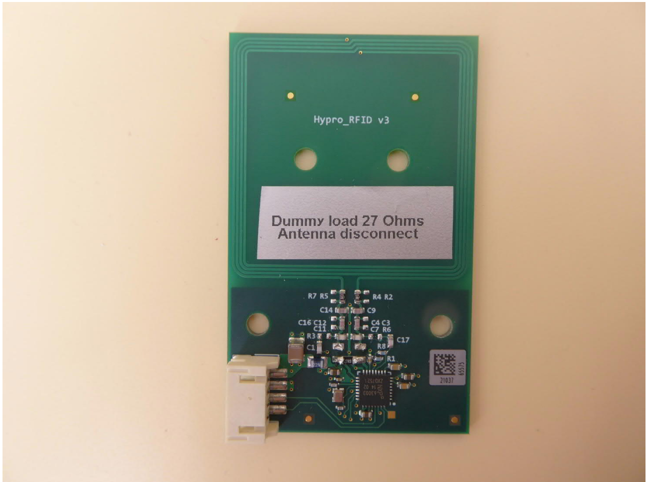
RFID PCB with dummy load, detail view
