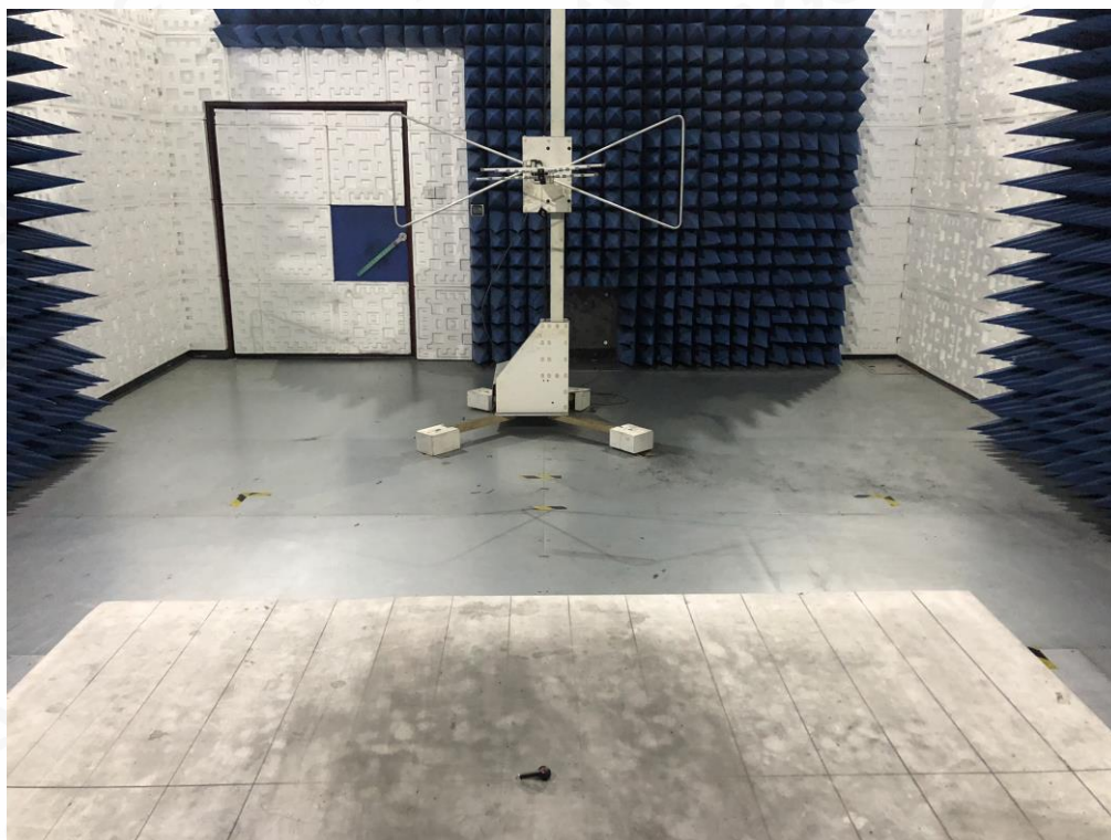
RADIATED EMISSION TEST SETUP ABOVE 1GHZ
