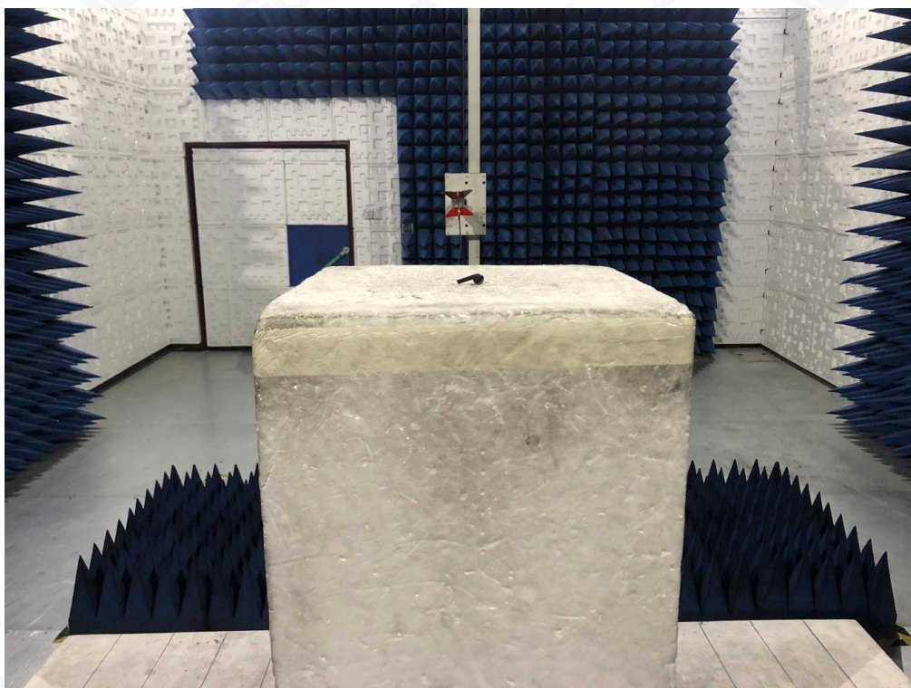
RADIATED EMISSION TEST SETUP ABOVE 1GHZ
