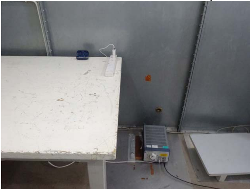
Measurement of Conducted Emission Test Set Up
