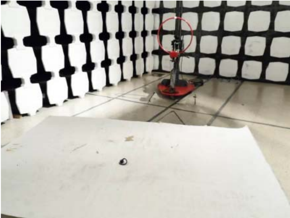
Measurement of Radiated Emission Test Set Up
