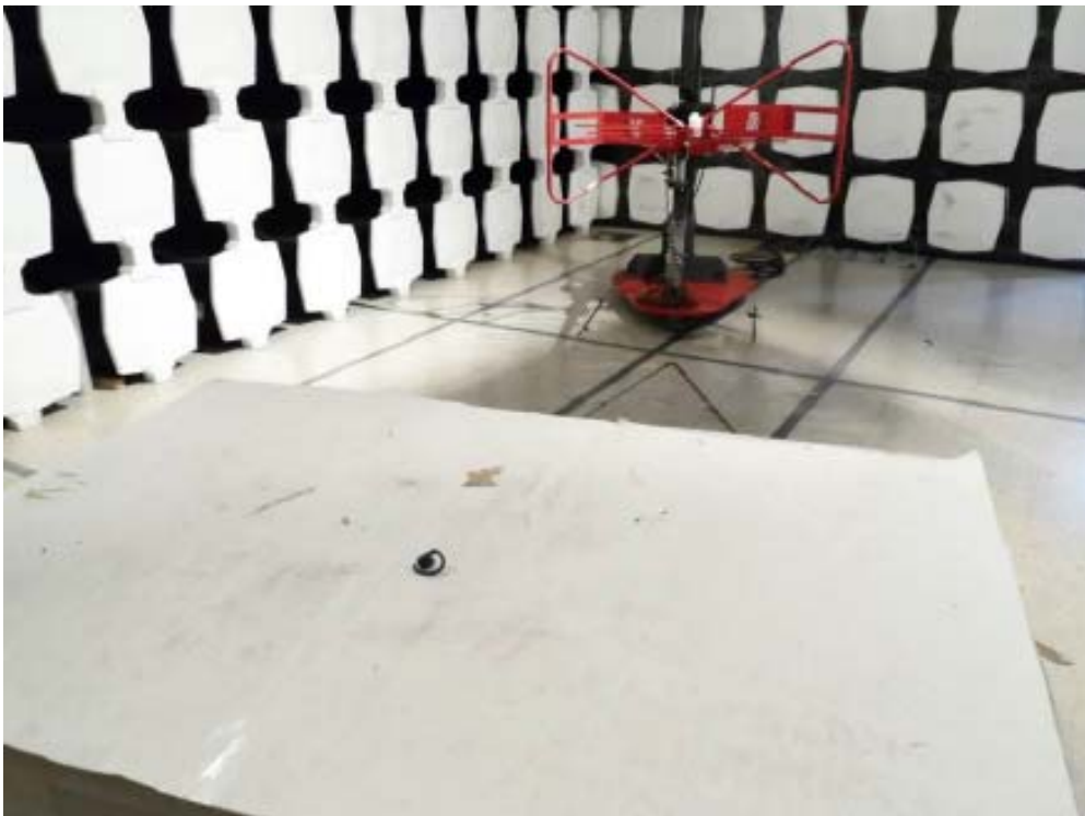
Measurement of Radiated Emission Test Set Up
