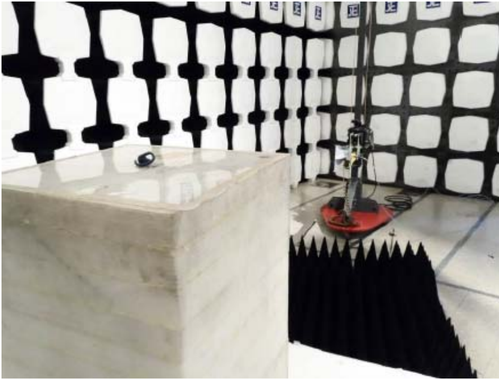
Measurement of Radiated Emission Test Set Up
