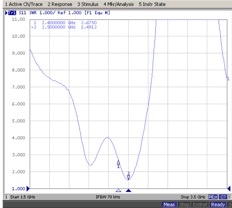
VSWR parameter in sample antenna tested in free space
