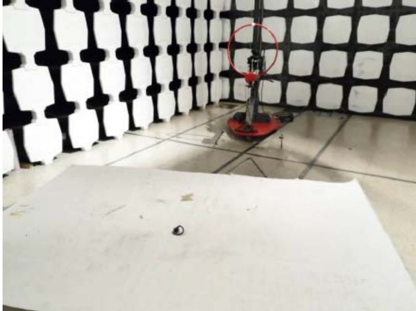
Measurement of Radiated Emission Test Set Up (9kHz – 30MHz)
