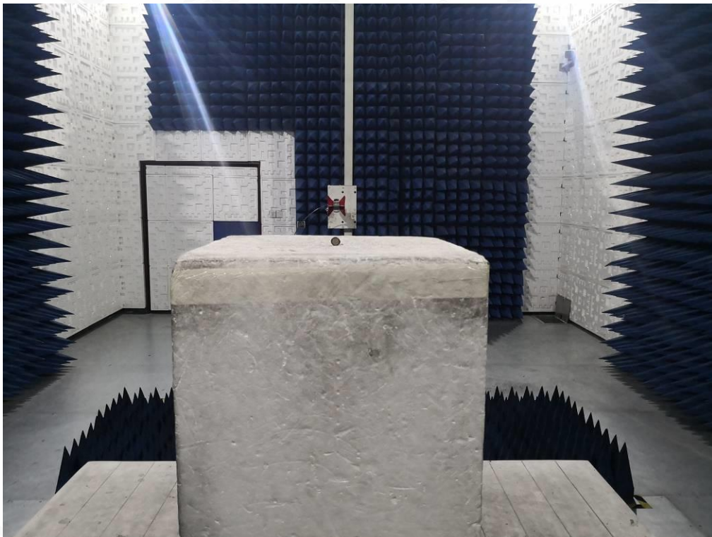
RADIATED EMISSION TEST SETUP ABOVE 1GHZ
