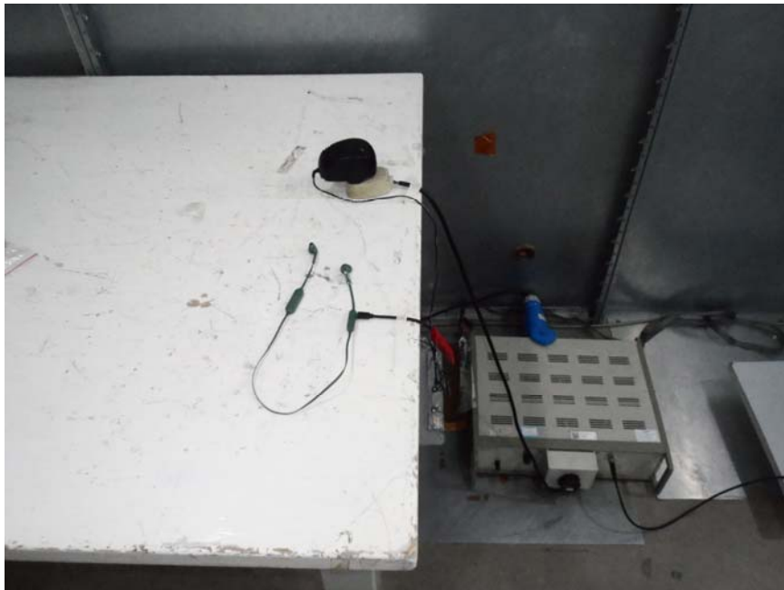
Measurement of Conducted Emission Test Set Up
