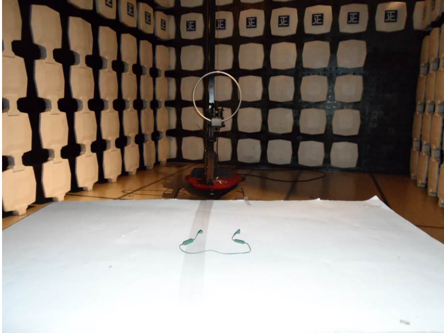
Measurement of Radiated Emission Test Set Up
