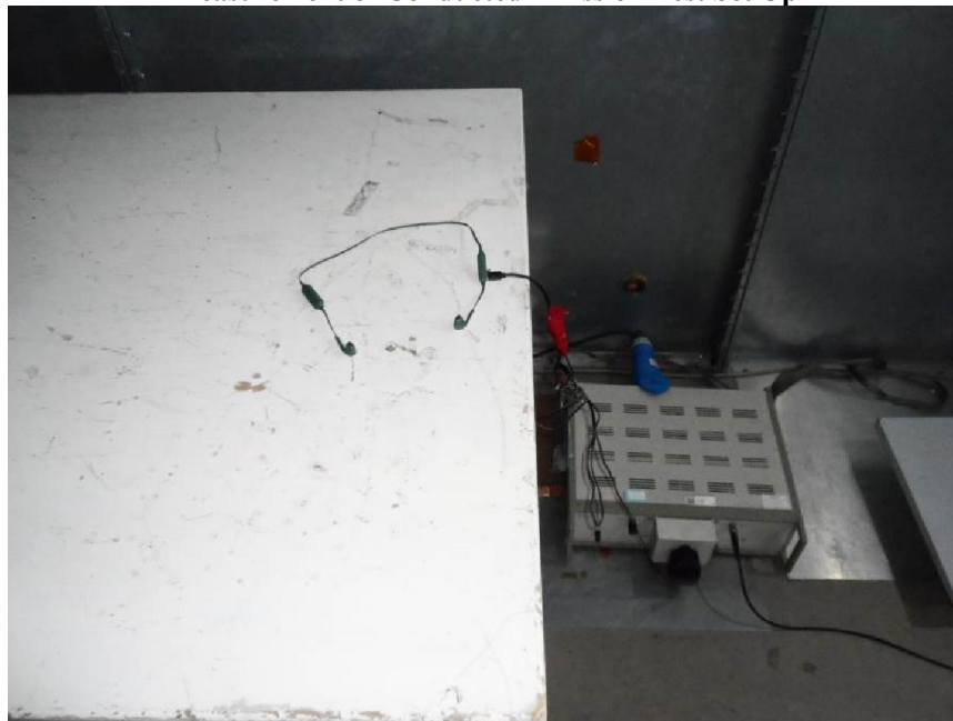
Measurement of Conducted Emission Test Set Up
