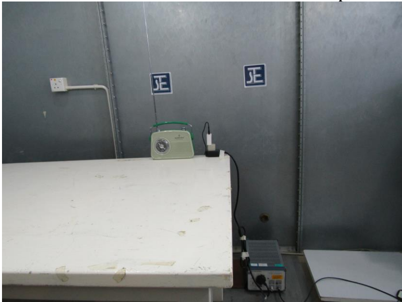
Measurement of Conducted Emission Test Set Up
