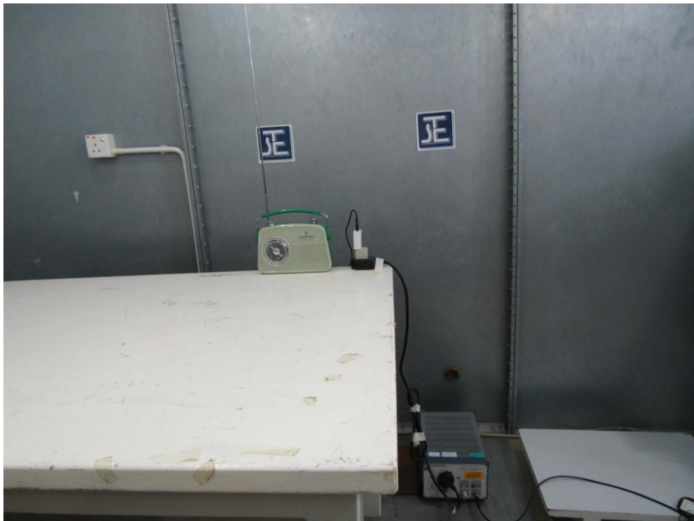
Measurement of Conducted Emission Test Set Up
