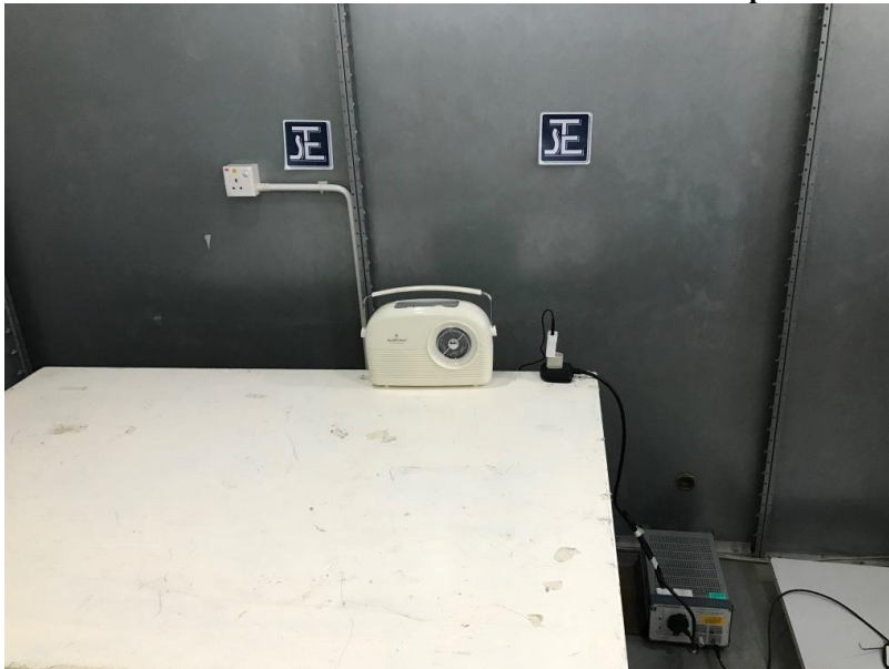
Measurement of Conducted Emission Test Set Up
