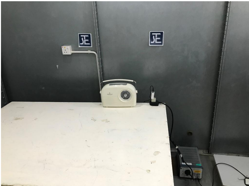
Measurement of Conducted Emission Test Set Up
