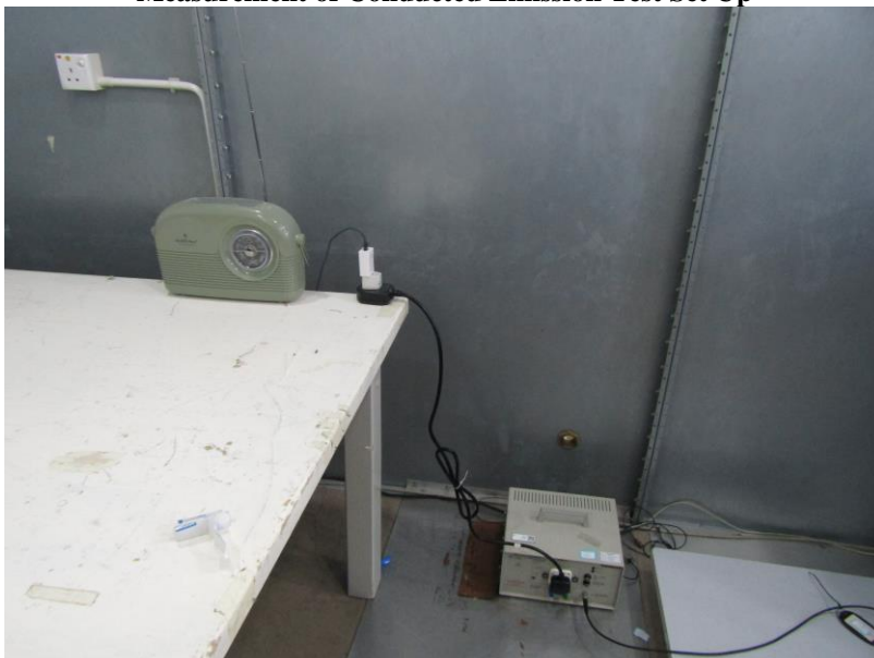
Measurement of Conducted Emission Test Set Up
