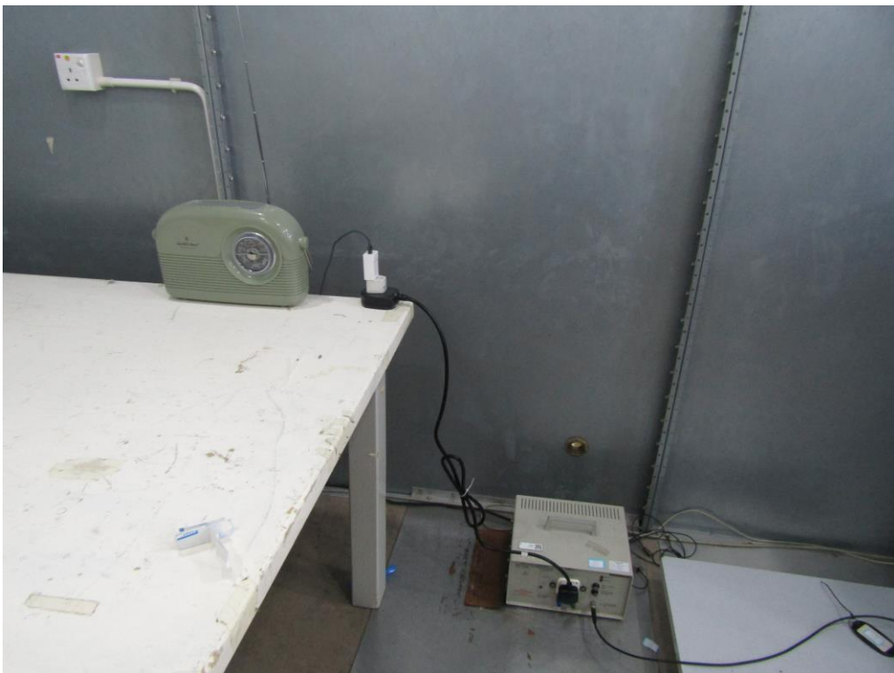
Measurement of Conducted Emission Test Set Up
