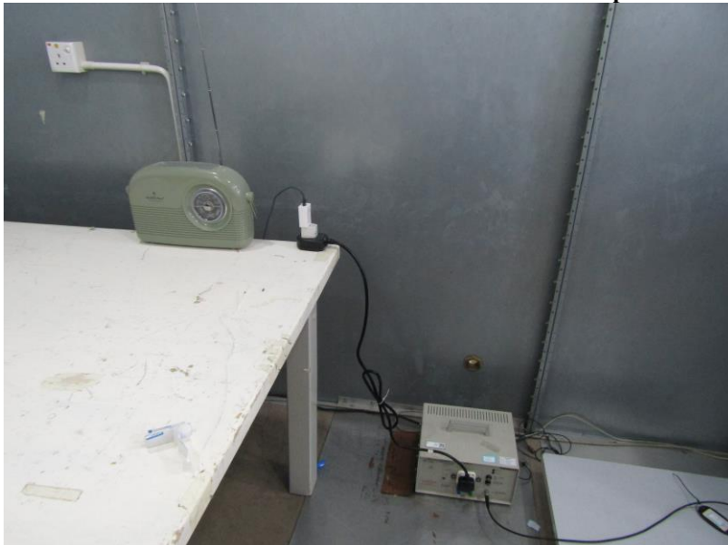
Measurement of Conducted Emission Test Set Up
