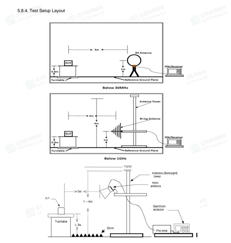
Above 18 GHz shall be extrapolated to the specified distance using an extrapolation factor of 20 dB/decade form 3m to 1m.
