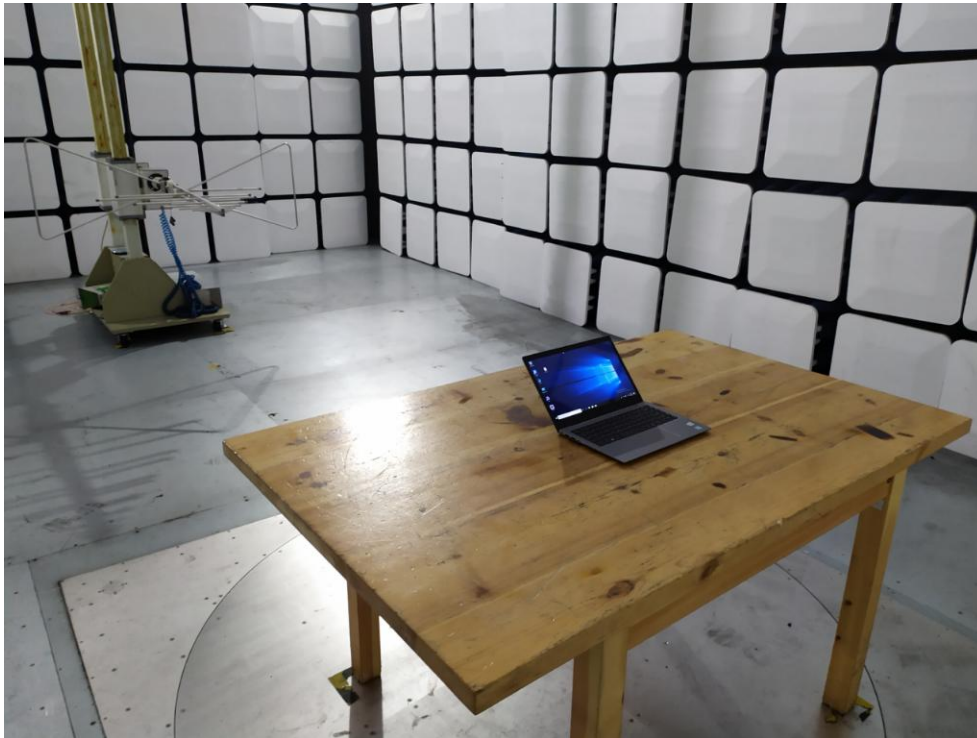
Photo of Radiation Emission Test
