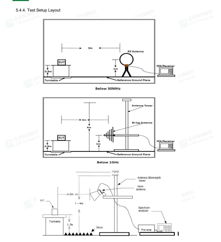
Above 18 GHz shall be extrapolated to the specified distance using an extrapolation factor of 20 dB/decade form 3m to 1m.
