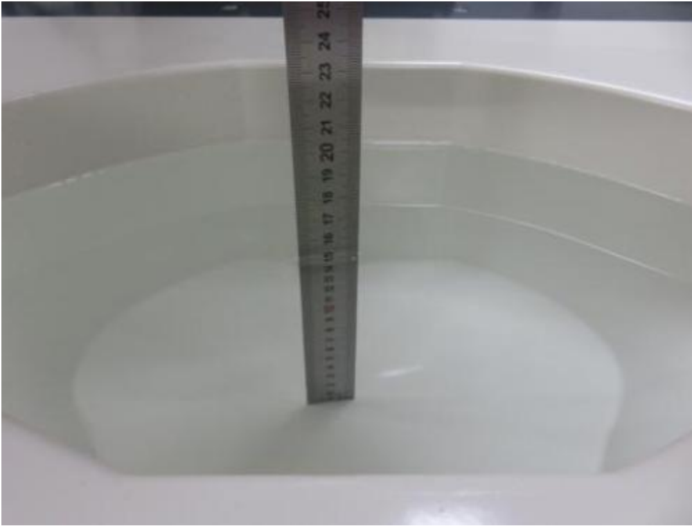
Photograph of the depth in the Body Phantom (5800MHz, 15.4cm depth)
