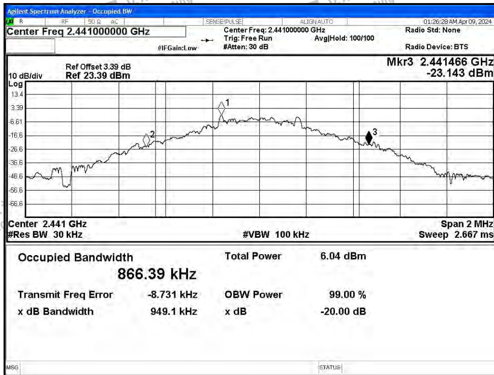
-20dB Bandwidth NVNT 1-DH5 2441MHz Ant1
