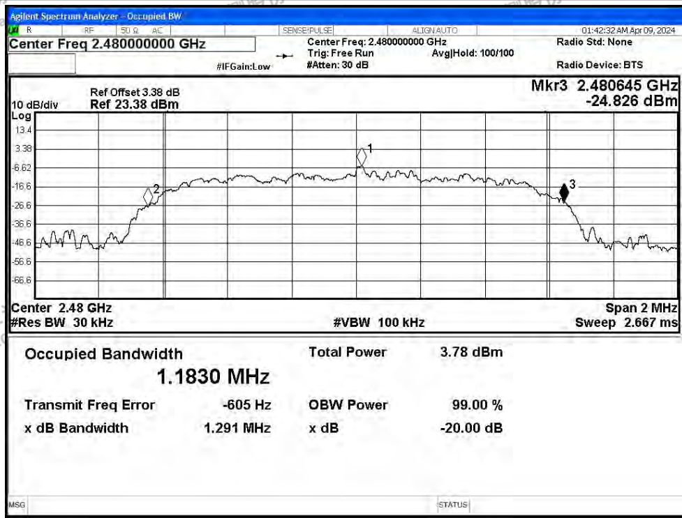
-20dB Bandwidth NVNT 2-DH5 2480MHz Ant1
