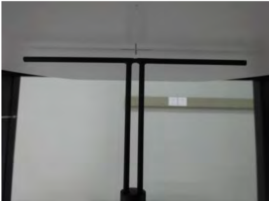
Photo of Dipole Setup
