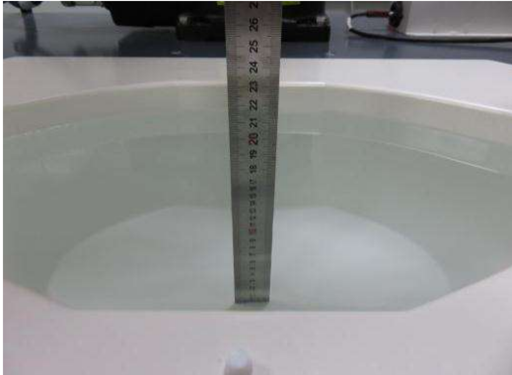
Photograph of the depth in the Body Phantom (5800MHz, 15.3cm depth)
