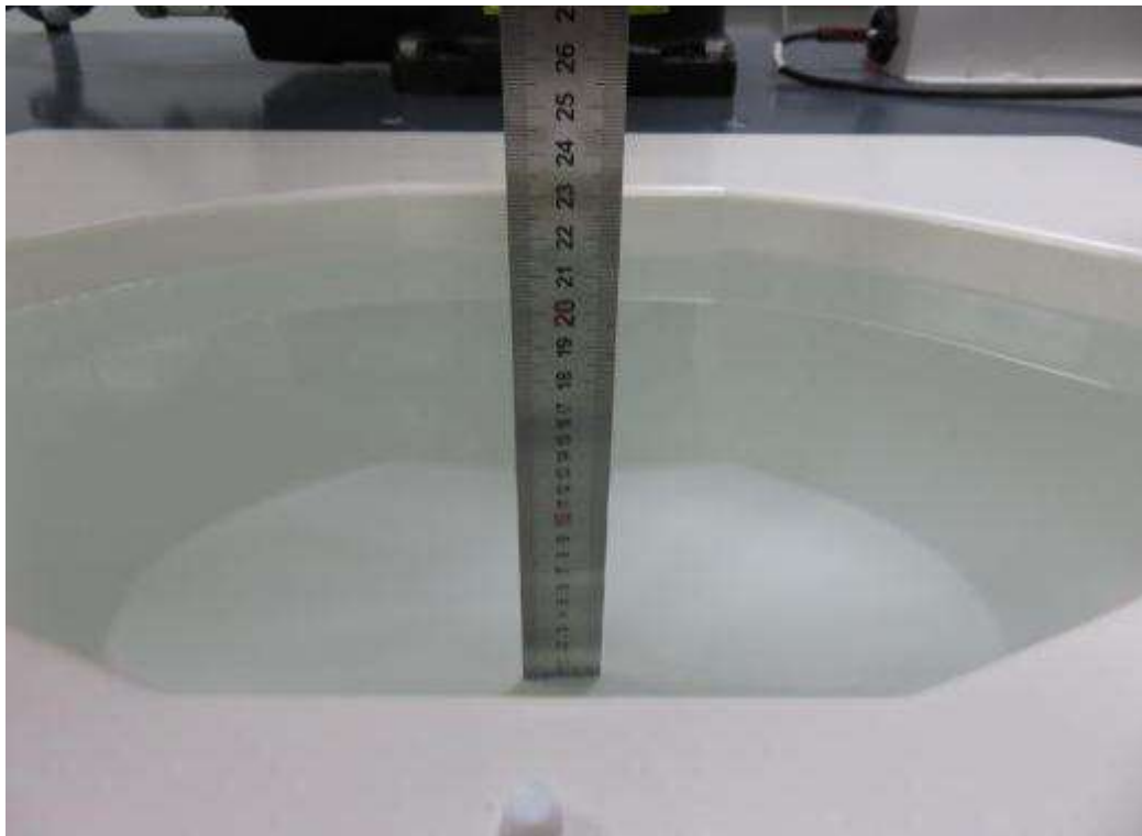
Photograph of the depth in the Body Phantom (5200MHz, 16.4cm depth)
