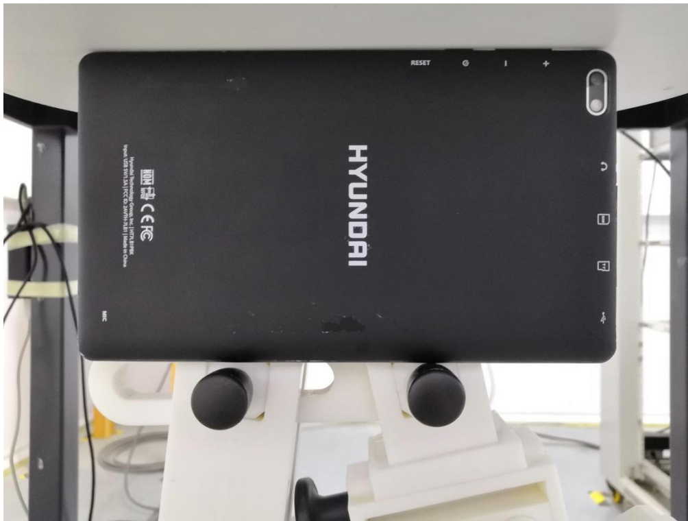
0mm body-worn Right Side Setup Photo (hotspot)
