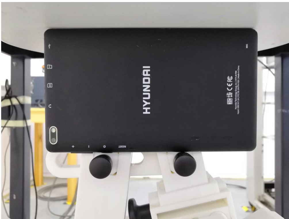
0mm body-worn Left Side Setup Photo(hotspot)
