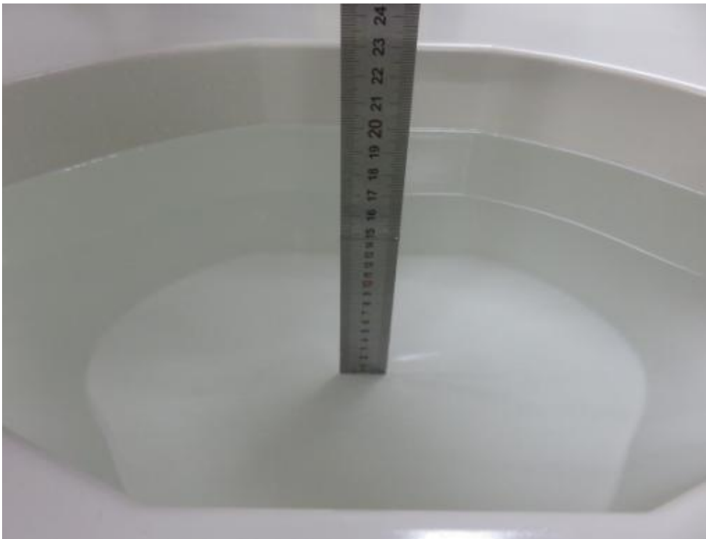
Photograph of the depth in the Body Phantom (2600MHz, 16.3cm depth)
