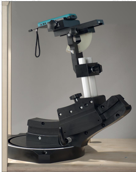
F-2. Device Holder for Transmitters
