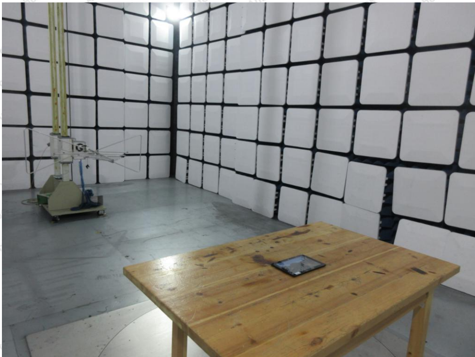
Photo of Radiation Emission Test
