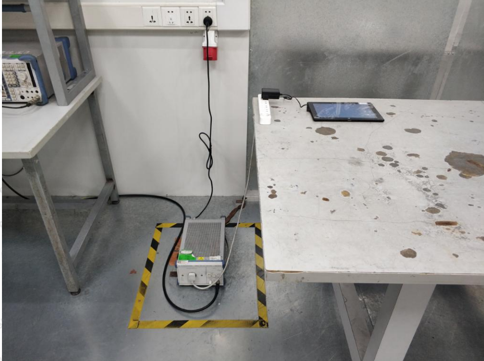
Photo of Conducted Emission Measurement
